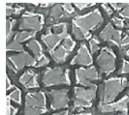
Figure 5. Electrode Surface after Coating
